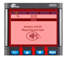
Position the (contactless enabled) card or device around the screen area of the terminal for a few seconds until a 'beep' sound confirms the card has been read (the green contactless LEDs will incrementally light up as the card is being read).
