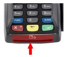
Insert the card (with the Chip of the card on top, facing towards you) into the Chip and PIN card slot at the base of the terminal.
