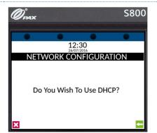
axept® S800 supports Dynamic Host Configuration Protocol (DHCP) which automatically obtains all network settings.
