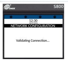
axept® S800 validates the network connection and communicates with the DHCP server to obtain an IP address and other network settings.
