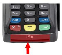
Alternatively, ask the cardholder to insert their card into (with the Chip of the card on top, facing towards you) into the Chip and PIN card slot at the base of the terminal.
