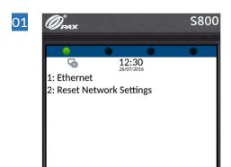
From the Network Settings menu, highlight 'Ethernet' using the and keys on the keypad (or press the key on the keypad) and press the key on the keypad to continue.
