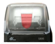
Insert the thermal paper roll into the axept® S800 terminal.
