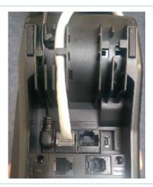
Once connected, run the cables through the cable management sections of the axept $^{\circ}$  S800 (as shown left).
