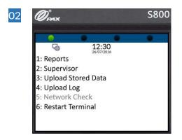
To initialise the upload, select option **3: Upload Stored Data** (Press the wey on the keypad).
